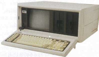
1982 FIRST COMMERCIAL SUCCESSFUL PORTABLE Compaq Portable PC with nine-inch monochrome monitor, 12.7kg.
